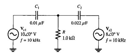
Step 1. Replace  $V_{s2}$  with its internal impedance (zero in this case), and find the current in R due to  $V_{s1}$ , as indicated in Figure 19–2.
