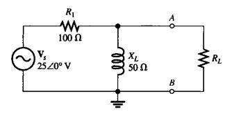
Solution First, replace  $V_s$  with its internal impedance (zero in this case), as shown in Figure 19-19. Looking in between terminals A and B,  $R_1$  and  $X_L$  are in parallel. Thus,
