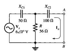
$I_n$  is the current through the short and is calculated as follows. First, the total impedance viewed from the source is
