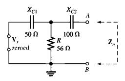
Looking in between terminals A and B,  $C_2$  is in series with the parallel combination of R and  $C_1$ . Thus,
