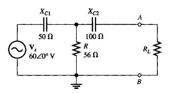
**Solution** Short the terminals A and B, as shown in Figure 19–34.
